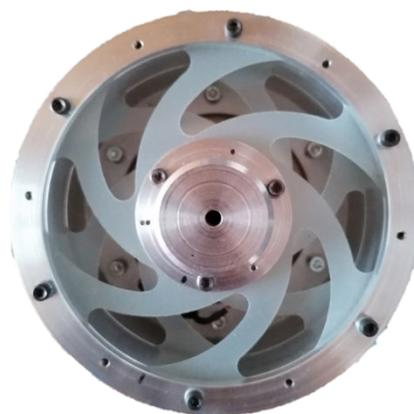
**Figure 8.** Presentation of the opposing installation of springs.
