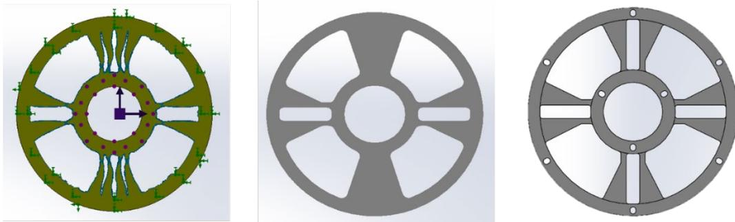
**Figure 4.** The process of processing the model obtained because of topology optimization.
