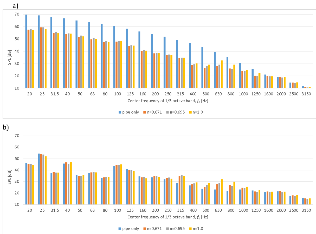
Figure 8. The time-averaged equivalent sound pressure levels, SPL [dB], in 1/3 octave bands for three analyzed helicoidal resonators placed in a cylindrical duct with air flow at a speed of 0 to 20 m/s without pink noise for two microphones positions in the distance of 1 m: a) in the pipe axis, microphone equipped with a nosecone, b) at an angle of 45 degrees, microphone equipped with a windscreen.
