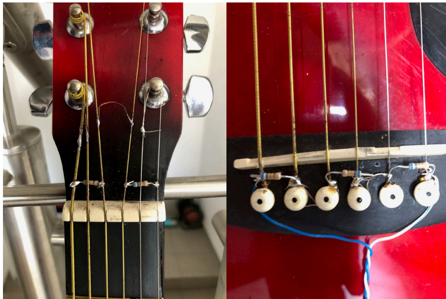
Figure 9. Connecting strings in series with resistors connected in parallel. On the left - by the nuts, on the right by the tailpiece.
