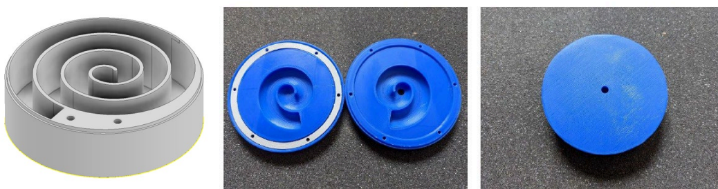
Figure 1. Examples of metamaterial structures based on the Helmholtz resonator.
