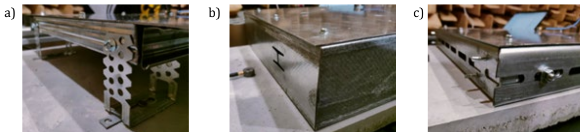
Figure 2. Ways of elements' connections, a) the CD-50 profile, b) the CD-100, c) the UA-50 profile.
