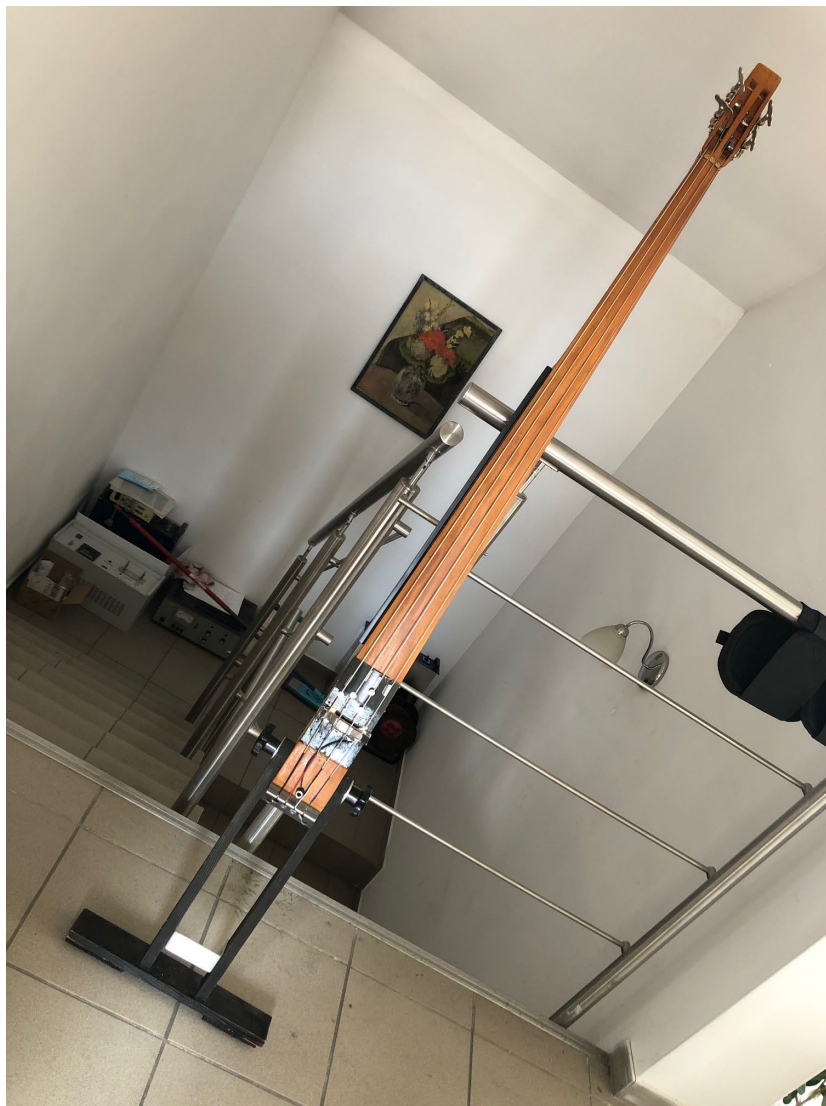
Figure 3. View of a double bass with 4 strings, one magnet and common contacts on the bridge and nuts.
