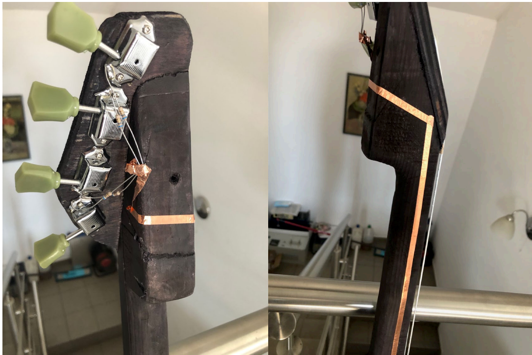
Figure 6. View of the passive system with strings connected in parallel and resistors by the nuts, on the left - view of 6.8 \Omega resistors connected in series with the strings, on the right - the signal cable from the strings.
