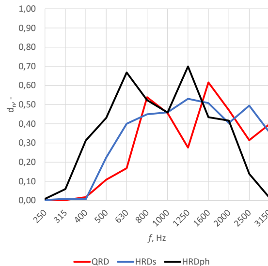
Figure 8. Comparison of the normalized diffusion coefficient of the optimized sound diffusers.
