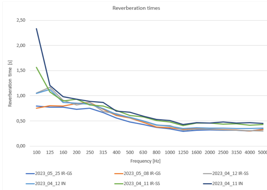
Figure 3. Reverberation time measurement results for subsequent measurements: IR-GS (impulse response, gun shot); IR-SS (impulse response, swept sine); IN (interrupted noise).
