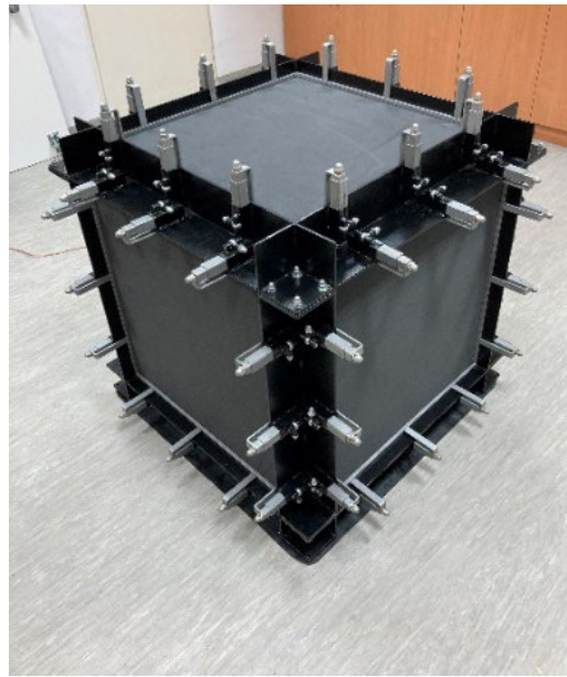
Figure 2. View of the enclosure with walls of XPE foam.
