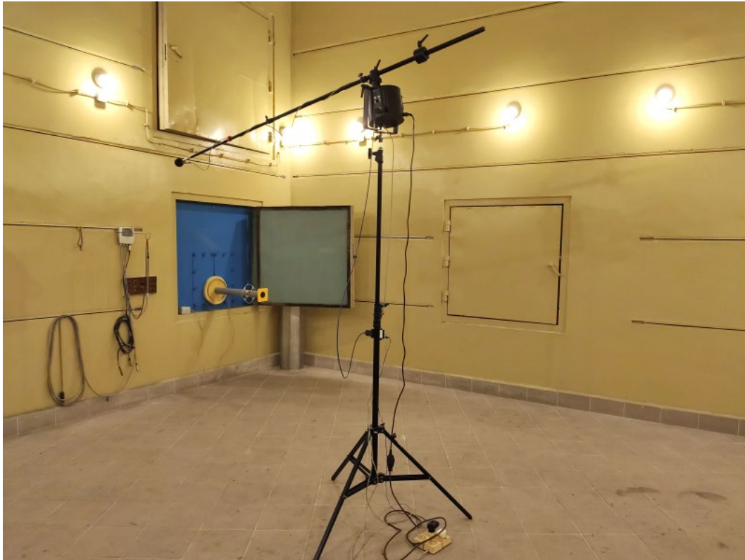
Figure 5. Reverberation chamber with visible fan outlet.
