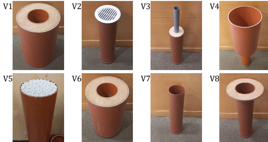
Figure 5. Waveguide open end modification variants: V1 – micro-perforated muffer (MPP), V2 – ventilation grille, V3 – sudden contraction, V4 – sudden expansion, V5 – tubes in open end, V6 – absorption muffer, V7 – open end without flange, V8 – open end with flange.
