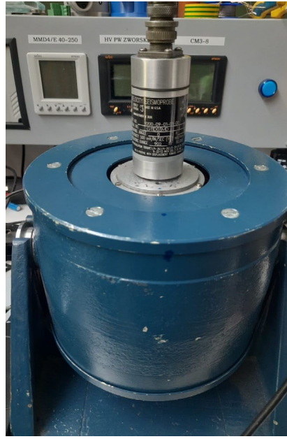
Figure 1. Vibration shaker with the Bently Nevada Seismoprobe transducer.
