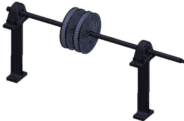
Figure 1. Computational model with finite elements mesh.
