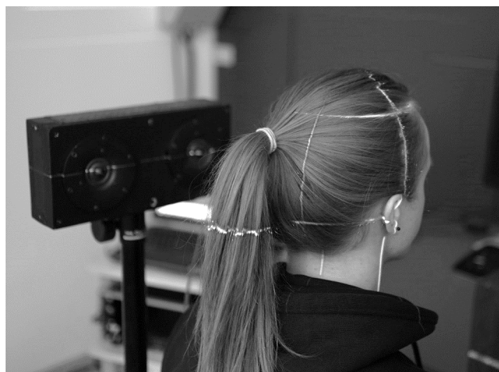
Figure 2. Positioning the speakers using laser levels.
